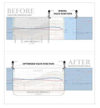
In this case example, the conductivity sensor was previously used in cream push-out, however it was inaccurate and reacted slowly to the cream/water interface, leading to losses of 500 liters of product in each push-out. With Collo, the optimal timing prevents losses. Cream is one of the costliest dairy products to produce and is also very costly to dispose of as waste.
