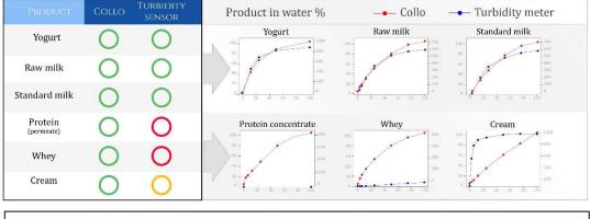
One of the key benefits in Collo s dielectric sensors is that the technology works with any liquid. Unlike turbidity sensors, it can accurately detect transparent, opaque and thick liquids, like whey concentrate or cream, from water, in addition to other milk-based and non-milk liquids.
